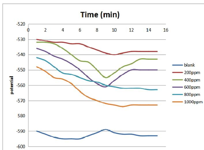
Fig. 1. Variation in open circuit potential (OCP) with time record for mild steel in 1.0 M  $\text{H}_2\text{SO}_4$  in the absence and presence of various concentrations of guar gum inhibitors at 298 K
