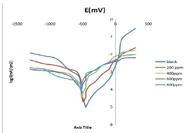
Fig. 2. Potentiodynamic cathodic and anodic plots of mild steel in 1.0 M  $H_2SO_4$  in the presence and absence of various concentrations of guar gum inhibitors at 298 K
