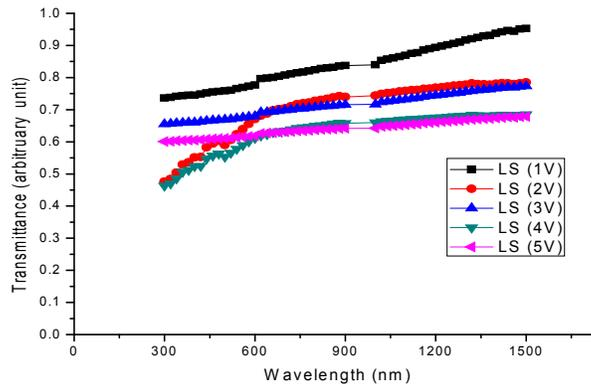
**Fig. 2. Plot of transmittance as a function wavelength**
