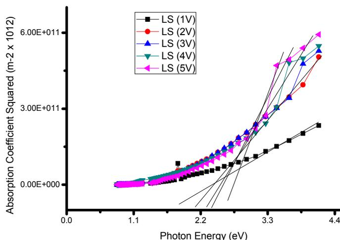
**Fig. 9. Plot of absorption coefficient square as a function of photon energy**
